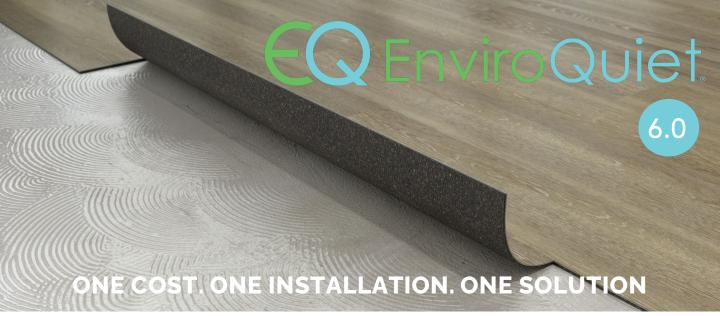
EnviroQuiet 6.0 is commercial grade 3mm LVT factory laminated to a 3mm thick acoustical underlayment, so it can be purchased and installed as one fully integrated product. With 5 patents worldwide, this formula provides an all-inone economical flooring solution that can be paired with most of our stunning wood or stone visuals
