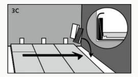
The diagrams indicate where the Rigid Hybrid panels are clicked together by angling up and down or where they are tapped together flat. Follow the diagrams precisely. See diagrams 4.1 > 4.16
